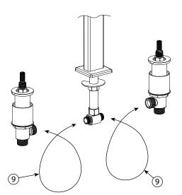
Connect stainless steel flex lines (9) from valve outlets to spout tee (7). Flex lines should be looped as shown in diagram. FLEX LINES MUST NOT BE KINKED. Adjust valves and or spout teeto eliminate any kinking in the flex lines. Install escutcheons onto the valves and hand tighten. DO NOT OVER-TIGHTEN. Install handles onto valve stems.
